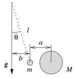
How far—due to the gravitational attraction of the Lead ball—does the pendulum ball move from its equilibrium position? Compare the distance it moves with the size of a typical atom (about  $10^{-10}$  m).
